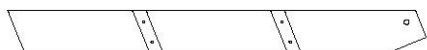
E02 | RAIL D'ÉCHELLE - W4L13970 (x3) | 1 3/8 po x 3 3/8 po x 32 3/4 po (36 x 86 x 831)
