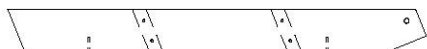
E03 | RAIL D'ÉCHELLE - W4L13973 (x3) | 1 3/8 po x 3 3/8 po x 32 3/4 po (36 x 86 x 831)
