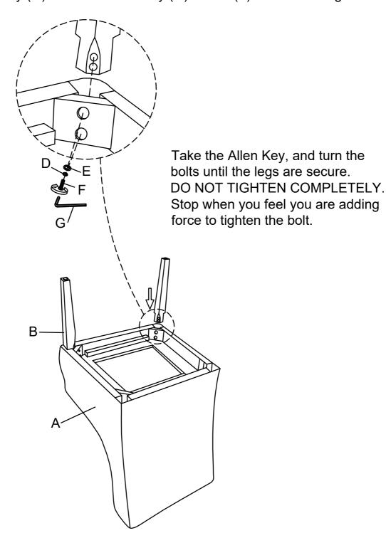
Attach Back Leg (C) to the Chair Body (A) using Bolt (F), Lock Washer (D) and Flat Washer (E) on both holes of Chair Body (A) by Allen Key (G). Turn the Allen Key (G) in Bolt (F). But not too tight.
