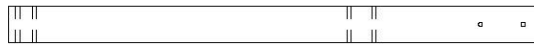
SP01 | SUPPORT DE POUTRE DE BALANÇOIRE - W4L16462 (x1) | 3 3/8 po x 3 3/8 po x 50 po (86 x 86 x 1 269)
