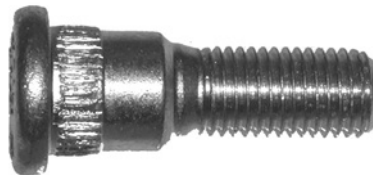
561-371 M12 x 1.5 x 43.8mm Knurl diameter: 17mm
