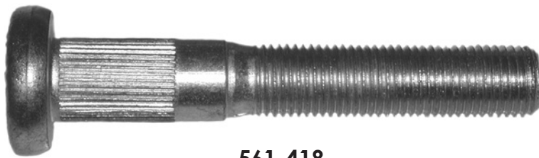
561-418 M14 x 1.5 x 91mm Knurl diameter: 15.7mm
