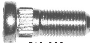
561-102 M12 X 1.25 x 32mm Knurl diameter: 12.9mm
