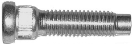
561-390 M12 x 1.75 x 51mm Knurl diameter: 14.73mm
