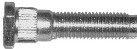
561-416 M12 x 1.5 x 52mm Knurl diameter: 14.8mm
