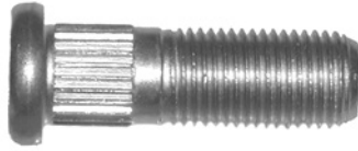
561-175 M12 x 1.25 x 38mm Knurl diameter: 12.24mm
