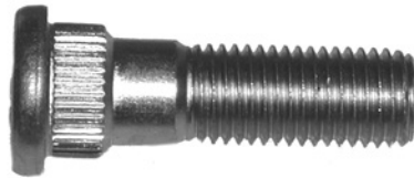
561-370 M12 x 1.5 x 44mm Knurl diameter: 15.8mm
