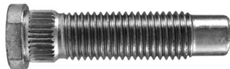
561-492 M12 x 1.5 x 48.3mm Knurl diameter: 12.84mm
