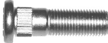
561-100 M12 x 1.25 x 39mm Knurl diameter: .12.9mm
