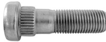
561-401 M12 X 1.25 x 42mm Knurl diameter: 14.43mm
