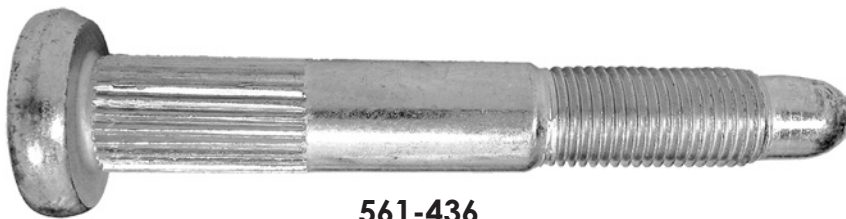
561-436 M14 x 1.5 x 104mm Knurl diameter: 16mm
