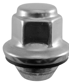
559-310 M12 x 1.25 21mm Hex 34mm Height Dometop Capped
