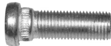
561-413 M14 x 1.5 x 43mm Knurl diameter: 15.7mm
