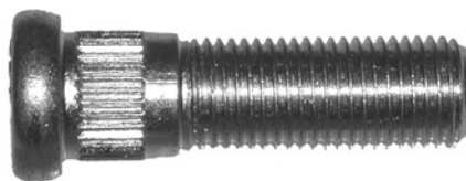
561-410 M14 x 1.5 x 49mm Knurl diameter: 15.7mm
