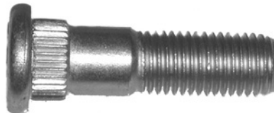
561-369 M12 x 1.5 x 46mm Knurl diameter: 15mm
