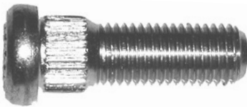
561-122 M12 x 1.5 x 36mm Knurl diameter: 14.3mm
