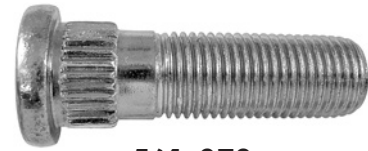
561-378 M12 x 1.25 x 42mm Knurl diameter: 14.35mm
