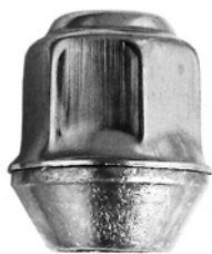
558-070 7/16-20R 3/4" Hex 1-1/8" Height Stainless Steel Capped
