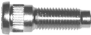
561-248 M12 x 1.5 x 43mm Knurl diameter: 14.5mm
