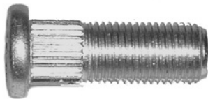
561-174 M12 X 1.25 x 34mm Knurl diameter: 12.24mm
