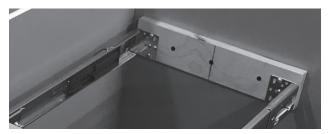
Line the front of the slide up with the edge of the face frame. Using 3. the front hole of the cabinet member, predrill a hole using a 1/8" drill bit. Secure each cabinet member to the face frame of the cabinet using one #6 x 1/2" screw (included) per side.
