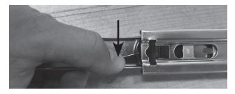
Slide the back of the cabinet member into the brackets you 2. installed on your cleat board.
