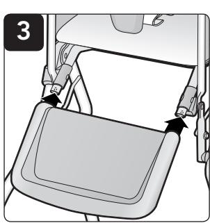
**4 Tray:** Depress side handles underneath tray and slide tray onto arm rests (**Figure 4**).
