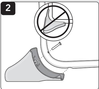
**3 Footrest:** Slide footrest onto high chair frame until pins "click" into place and pin protrudes through each hole (**Figure 3**). TIP: Squeeze pins while sliding on footrest.
