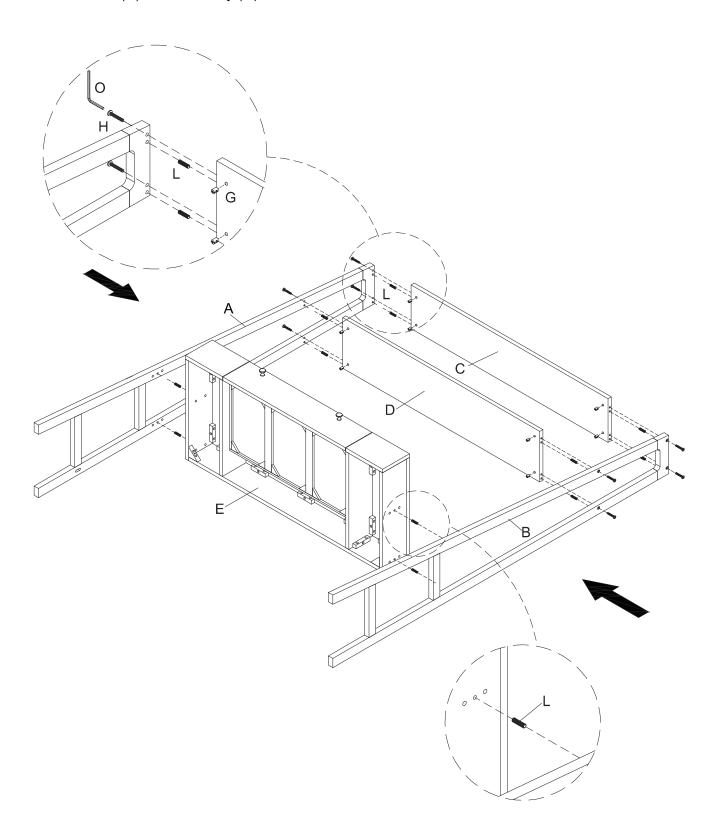
Fix Left & Right Leg Frame (A & B) with Desk (E) using Allen Bolt (I), Lock Washer (K) and Flat Washer (J) with Allen Key (O).
