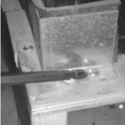
Image 1: Removing bracket from skid
