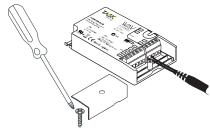
2. Use #2 Phillips to loosen screw and remove cover from WAV RGB Smart Receiver. Use the flat head from the multi-bit screwdriver to loosen terminals marked (B-), (G-), (R-), and (+).
