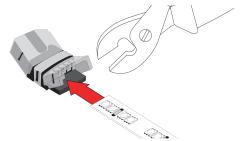
5. Peel back 1/2" of adhesive protector from back of RGB Tape Light; insert end of Tape Light all the way into short side of connector. Close cap and press gently with pliers to secure connection.
