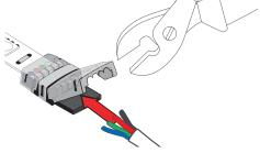
6. Leaving insulation intact, insert the 4 colored RGB wires into corresponding wire channel on long side of connector. Close cap and press gently with pliers to secure connection. The connector will cut through insulation to make contact.
