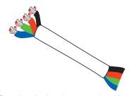
1. Cut a length of 4-wire connection wire to run from WAV RGB Smart Receiver to Tape Light location. On the end of the wire going into the receiver, strip 3/4" white sheathing, then strip 1/4" insulation from end of wire, twist each wire, and fold stripped wires in half. DO NOT strip ends of wire that will go into the connector.
