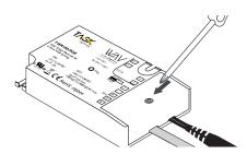
4. Replace the WAV RGB Smart Receiver terminal cover, ensuring wires are not pinched too tightly. Tighten Screw.
