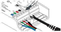
3. Insert one end of stripped 4-wire connection wire into their corresponding terminals, Blue wire to (B-), Green wire to (G-), Red wire to (R-), and Black wire to (+). Tighten screws.
