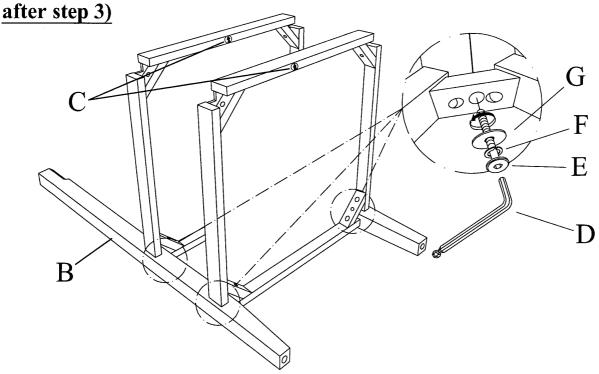
2 Attach the other Leg (B) to Shelf (C) using JCBC Bolt (E), Spring Washer (F) and Flat Washer (G).
