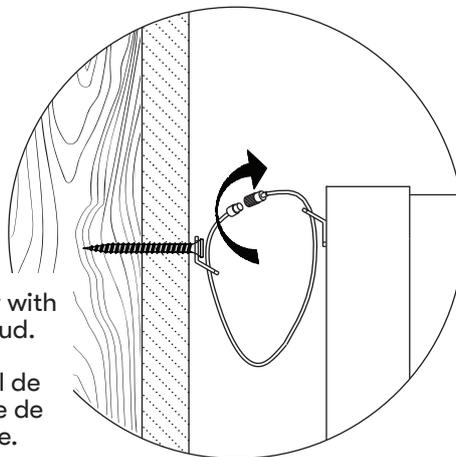
Put the male end of the steel cable through each bracket, Securely connect both ends together by turning the female connector clockwise.
