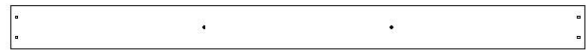
M01 PLANCHE DE PLANCHER - W4L16120 (x1) 5/8 po x 3 3/8 po x 44 7/8 po (16x86x1140)
