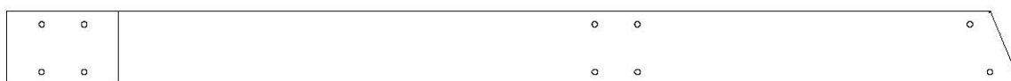
G03 RAIL AU SOL - W4L16132 (x1) 1 po x 5 1/4 po x 71 3/8 po (24x134x1814)
