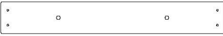
H75 PLANCHE DE FIXATION - W4L16159 (x1) 1 po x 3 3/8 po x 23 1/2 po (24x86x596)
