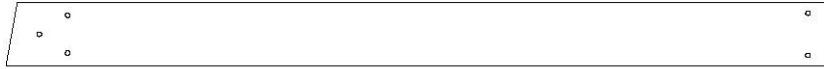
A74 POUTRE DE BALANÇOIRE 2 POSITIONS - W4L16167 (x1) 3 3/8 po x 5 1/4 po x 68 3/4 po (86x134x1745)
