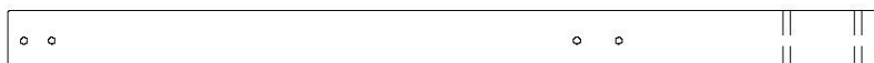
SP71 SUPPORT DE POUTRE DE BALANÇOIRE - W4L16168 (x1) 3 3/8 po x 3 3/8 po x 49 1/2 po (86x86x1256)
