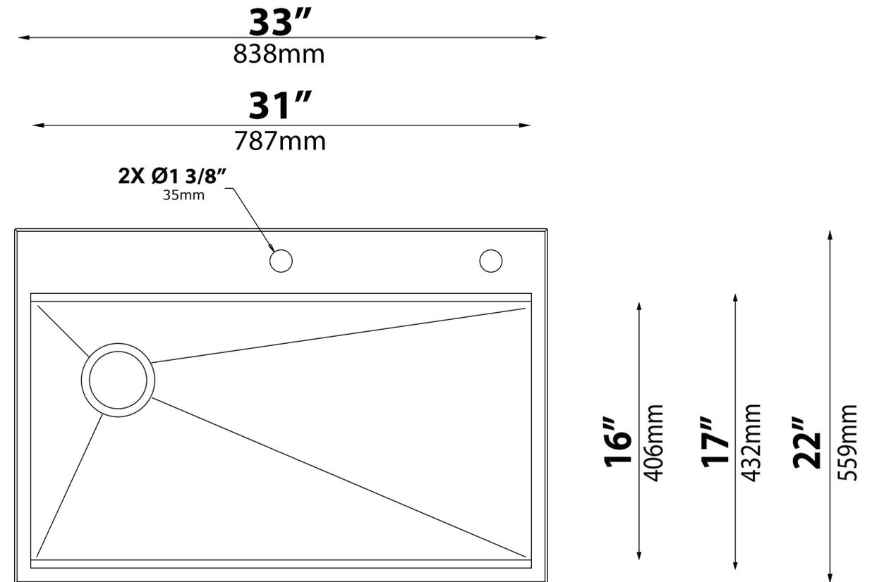
**NOTE:** Cutout template is provided as a guide **ONLY** and must be checked against actual sink to verify correct fit.
