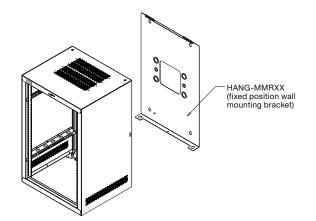
A Mounting Holes В Compatible With Part# Weight Capacity HANG-MMR10 16.0" [406.4] 20.58" [522.73] 150 lb. [68.04kg] MMR-1020 HANG-MMR12 24.08" [611.63] MMR-1220 19.5" [495.3] 150 lb. [68.04kg] HANG-MMR16 26.5" [673.1] 31.08" [789.43] 150 lb. [68.04kg] MMR-1620/MMR-1624 HANG-MMR18 MMR-1820/MMR-1824 30.0" [762] 34.58" [878.33] 150 lb. [68.04kg]
