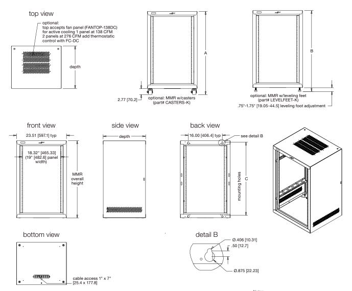
Notes: Direct to Wall Mount: 250 lbs [113.4kg] weight capacity Floor Standing: 250 lbs [113.4] weight capacity
