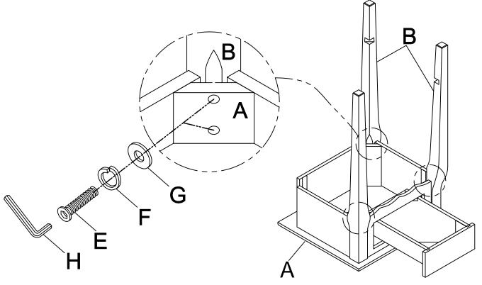
**2** Attached Shelf(C) to the Leg(B). Use Screw(D), on holes of Shelf(C). Attached the rest Leg(B) to the Table Top(A). Use Allen Bolt(E) Lock Washer(F) and Flat Washer(G) on holes of Table Top(A). Tighten the Allen Bolt(E) on Leg(B).
