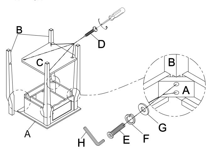
**3** Take out the drawer, and remove the handle at back side of drawer. Use bolt install the handle on front side.
