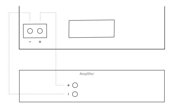
Note: when connecting, polarity shall NOT be reversed, as the reflected sound from the wall will be in phase with the top-boxes.
