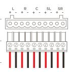
Observe polarity when making speaker connections!
