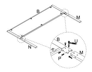
Attach the Headboard Stretcher (A) to Left Leg (M) and Right Leg (N), insert the Bolt (P), turn the Ratchet Tool (U) to tighten them.
