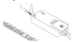
1. When pairing additional Zones to the same Controller, clear the memory on the new Receiver for the next Zone by pressing and holding the "Learn" button until the lights blink.
