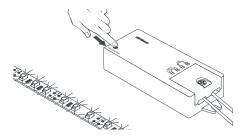
2. Each time a new Receiver is set up for the first time, clear the memory by pressing and holding the "Learn" button until the lights blink.
