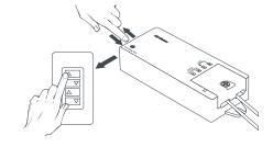
3. Very quickly, click and release the "Learn" button and, within 5 seconds, quickly click and release the "Up Arrow" button on the Controller for any of the Zones. When lights blink, Controller and Receiver are paired.
