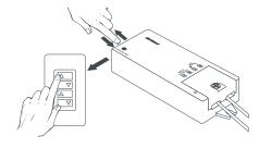
2. Very quickly, click and release the "Learn" button and, within 5 seconds, quickly click and release one of the "Up Arrow" buttons on the Controller for any of the Zones. When lights blink, Controller and Receiver are paired. Repeat process until Zones are paired as desired.
