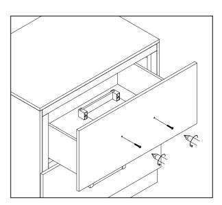
STEP 3: Place the handle on the outside of the drawer and screw from the inside of the drawer with a screwdriver. \*\* Attention: DO NOT OVER TIGHTEN THE SCREWS.
