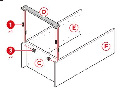
Attach the top panel assembly with four part 1 dowels and four part 3 cam locks.
