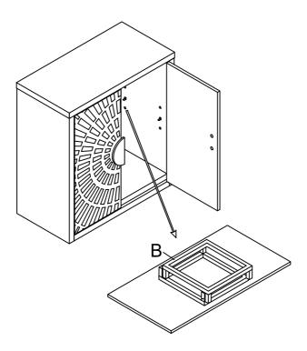
Insert Leg Frame (B) into Top Stretcher (C) and Bottom Stretcher (D) by using Flat Washer (G) and Small Bolt (E) with Allen Key (H).
