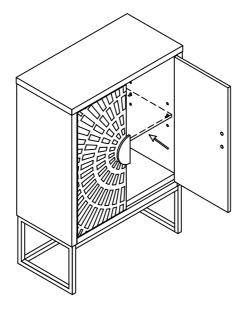
Remark: To prevent tip over, the product should be attached to the wall with Anti-Tipping Kit (J). Please read the individual AI for the Anti-Tipping Kit (J) thoroughly and install on the back of the product.
