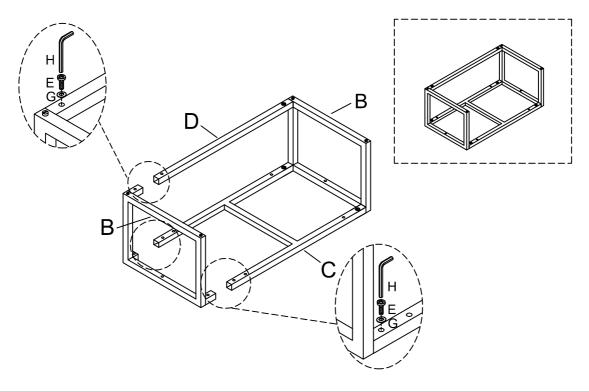
Attach the assembled frame to the bottom of Cabinet (A) by using Flat Washer (G) and Large Bolt (F) with Allen Key (I).
