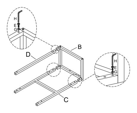
Insert Leg Frame (B) into Top Stretcher (C) and Bottom Stretcher (D) by using Flat Washer (G) and Small Bolt (E) with Allen Key (H).
