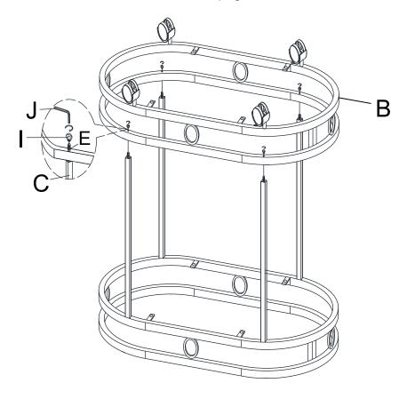
Attach Suction Cap (F) to Top Frame (A) and Bottom Frame (B) as shown.
