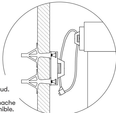
Loop provided 2 ties through both brackets and secure tightly.
