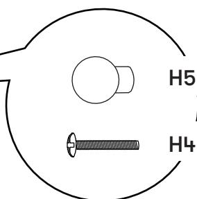
\* H5. Knob (x7) and H4. Knob bolt (x7) are pre-installed inside each drawer.
