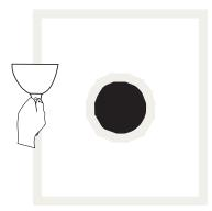
Secure sheetrock panel to the studs and apply mesh tape and joint compound to hide the installation seams. Make sure to apply joint compound up to the rim of the PB board.
