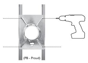
After determining the installation area for the speaker, secure the PB board to the wall studs while making sure that the inner rim of the PB extrudes away from the wall and not into the wall as shown in step 2.
