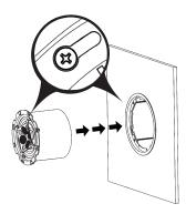
Depending on the model of speaker being installed, a bracket may need to be installed prior to speaker installation. If required perform this step now. (QXC bracket shown).
