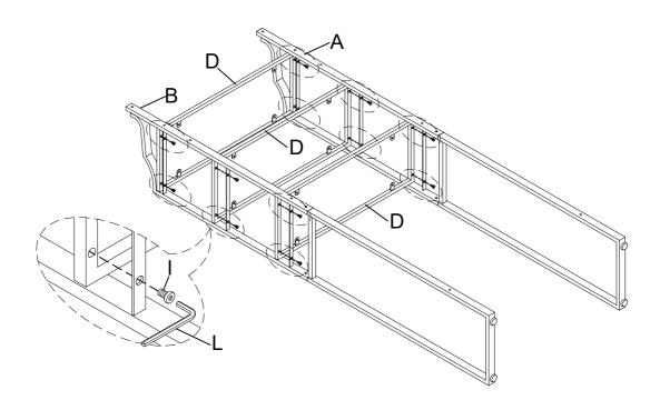
Assemble Cross Bar (E) to Side Upper Frame - LSF (A) & Side Upper Frame - RSF (B), using Bolt (I) by Allen Key (L) as below shown.
