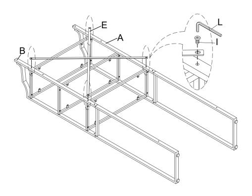
Assemble Upper Connect Bar (F) to Side Upper Frame - LSF (A) & Side Upper Frame - RSF (B), using Bolt (I) by Allen Key (L) as below shown.
