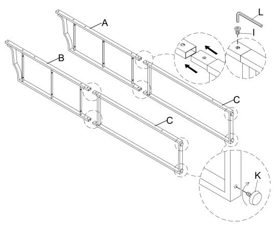
First, assemble Shelf Frame (D) to Side Upper Frame - LSF (A) & Side Upper Frame - RSF (B), using Bolt (I) by Allen Key (L) as below shown.
