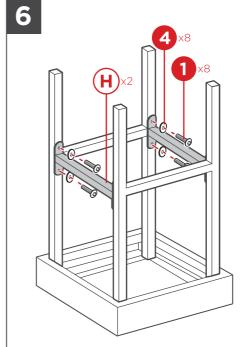
Attach two part H supports with eight part 1 screws and eight part 4 washers, four screws/washers per support.
