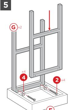
Attach two part G legs to the part F seat with four part 2 screws and four part 4 washers, two screws/washers per leg.
