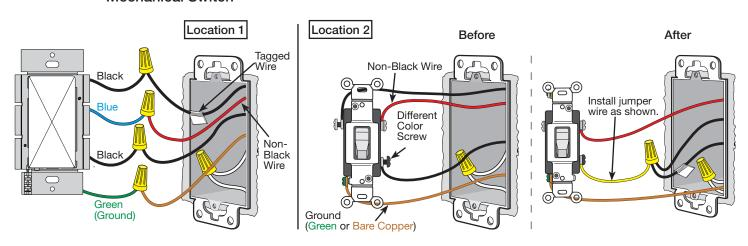
Note: If using a sensor switch, both ground wires must be connected for the sensor to operate.
