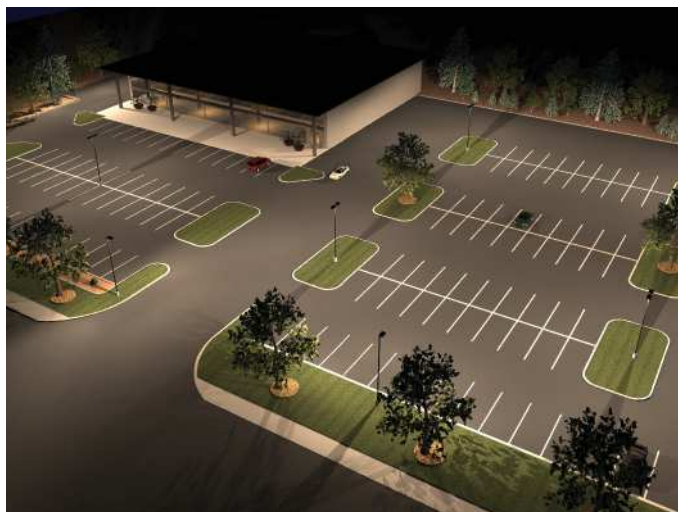
Prevail A40 LED 14 Fixtures = 2,002 Total watts
