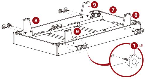
Lift the table assembly and flip it upright before returning it to your building surface. Do not tip the assembly or lean it on the legs, as this may damage the product.
