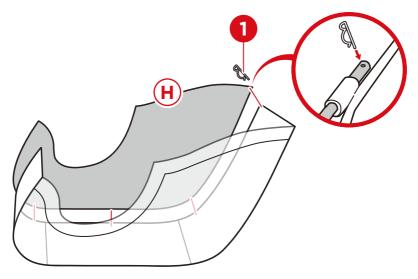
Insert the part J left runner and part K right runner and secure with two part one cotter pins and two part 3 zip ties, one on each side.
