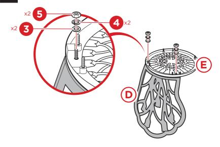
Attach four part F chair legs to the seat with eight part 3 washers, eight part 4 spring washers, and eight part 5 nuts.
