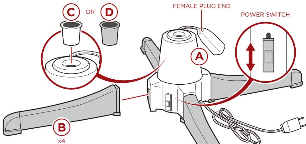
Slide four **part B legs** onto the **part A base**.
