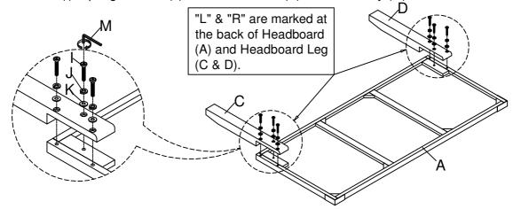
Attach Side Rail (E) to Headboard Leg - Left & Right (C & D) and Footboard (B) by hooking the Side Rail Brackets on the bolts (already on HB Legs & FB) and tighten all the bolts using Allen Key (M).
