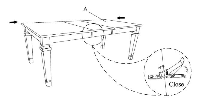
6 Unlock the latches underneath table top(A). Pull apart the table top(A) at both ends and take out the center leaf(B).
