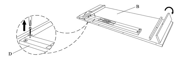
Place table top(A) upside down on soft surface. Align and fasten leaf support(D) to table slide on the table top(A). Using short bolt(J), small spring washer(K) and small flat washer(L) and tighten with small Allen wrench(I).
