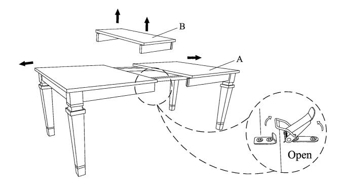
7 Fold the center leaf(B) apron. Keep the center leaf(B) underneath table top(A) and hang on the leaf support.
