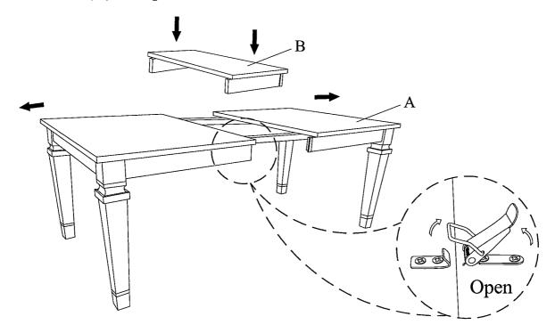
5 Push both ends together and make sure pin line up. Close the table top(A) tightly and lock all latches on the underneath of the table.
