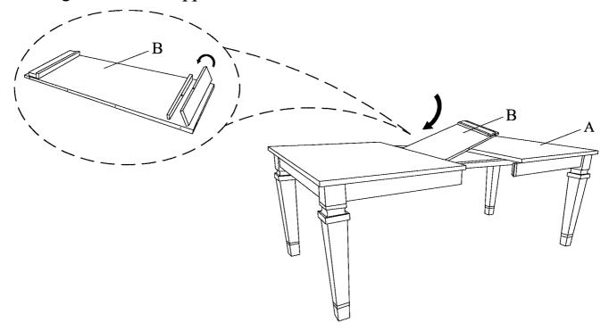
8 Push both ends together and make sure pin line up. Close the table top(A) tightly and lock all latches on the underneath of the table.
