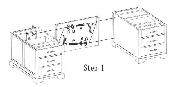
Step 1: Assemble the left and right bases and the center panel with Bolt (A), Lock Washer (B) and Washer (C) using wrench (F)
