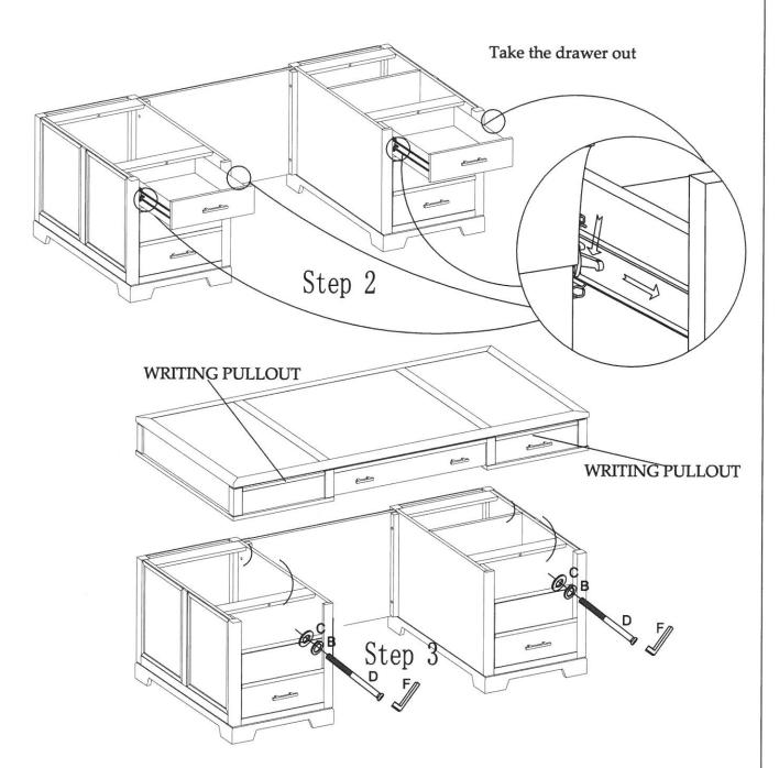
Step 2: Remove the upper drawers in both pedestals - Open drawer fully to expose the release levers in the center of the drawer slide. Push the lever on the left side up, and the lever on the lever on the right side down to release drawer. With levers pushed gently tug the drawer out of the desk
