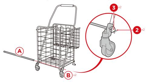
Slide a part A axle through the other side of the frame. Slide two part 1 washers and two part C rear wheels onto the axle.
