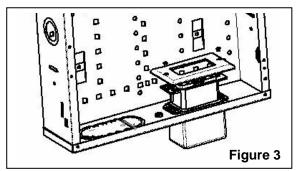
Use a Surge Protected Outlet Kit and one or two Power Strip Modules, PN 364266-01. Or, use a Duplex Outlet Power Kit, PN 364569-01, with one or two Surge Protected Power Strip Modules, PN 364771-01. See Technical Bulletin TB-0010.
