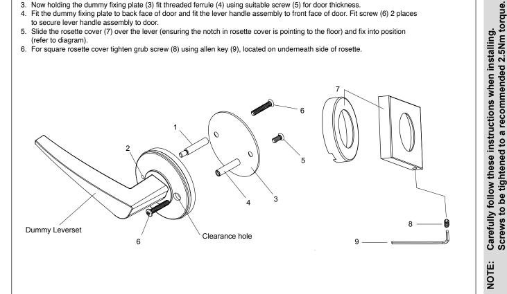
Note: Notch in round rosette cover or grub screw hole in square rosette cover should point to floor - refer diagram.
