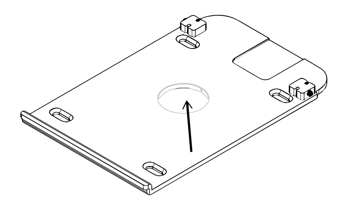
4. Option B, Run the cable out the back of the WedgeMount making sure to remove the cable channel cover.
