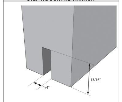
Mortise a 1/4" wide x 13/16" deep groove in the center bottom of the door to use with the floor-mounted door guide. This will prevent the door from swinging in and out and ensure smooth travel side-to-side.
