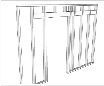
**NEW CONSTRUCTION:** Wood blocking can be installed inside the wall in a new construction.
