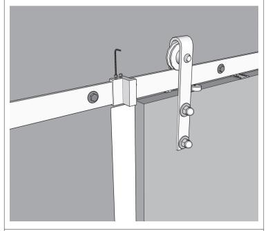
Adjust the door stops accordingly using an Allen Key (not provided).
