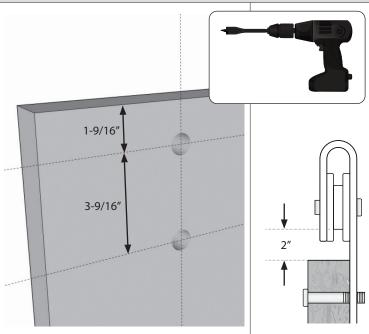
Determine your strap location. Position each strap against the front of the door a minimum of 2" from the edge or center of the stile.
