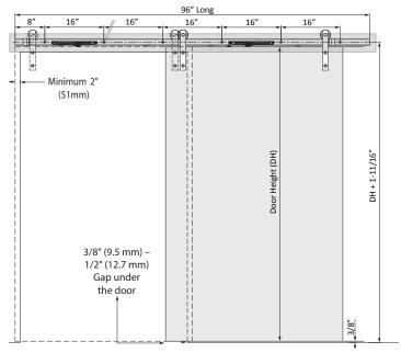
When installing into drywall, a piece of solid wood blocking is required to be mounted inside or outside of the wall before proceeding with the track installation. Position the solid wood blocking with track by measuring up from the door height (DH) + 1-11/16" to the center of the track. This allows a 3/8" - 1/2" gap at the bottom. For outside wall blocking, ensure it is level and leave a minimum of 2" from the end of the blocking to the side of the opening.
