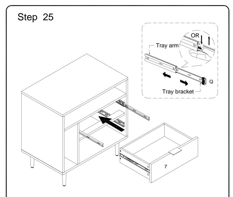
Put tray bracket (Q) into tray arm as per diagram .
