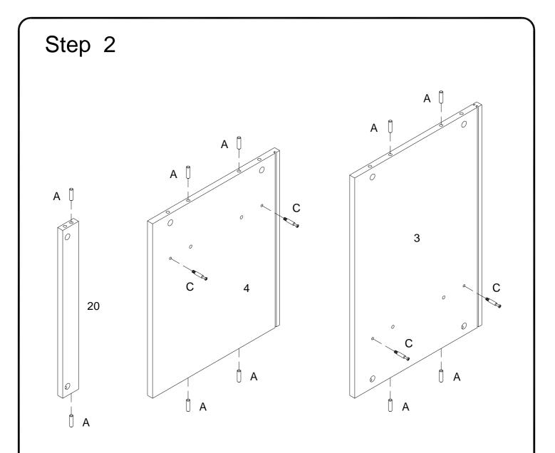
Insert wooden dowel (A) into parts (3,4,20), using cam bolt (C) secure parts (3,4) with Philips head screwdriver as per diagram.
