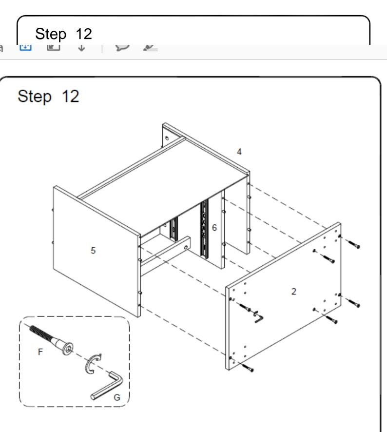
Using bolt (F) secure part (2) into parts (4,5,6) with hex key (G) as per diagram.
