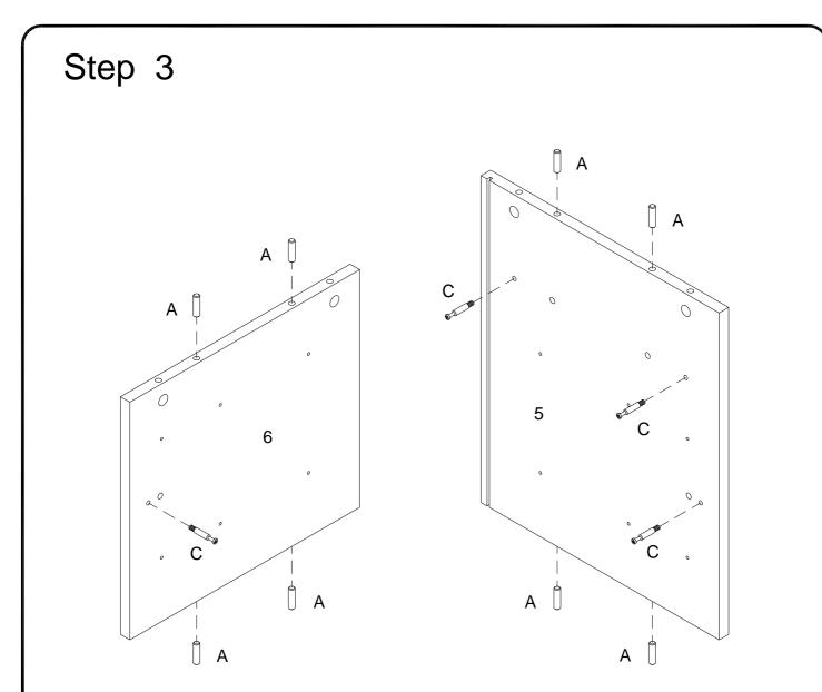
Insert wooden dowel (A) into parts (5,6), using cam bolt (C) secure parts (5,6) with Philips head screwdriver as per diagram.
