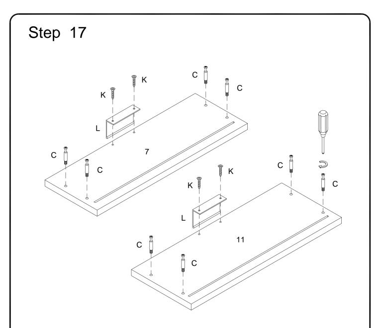
Using cam bolt (C), screw (K) secure knob (L) to parts (7,11) with Philips head screwdriver as per diagram.
