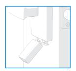
9V battery connections are located in a slide down tray under the front of the outside escutcheon.
