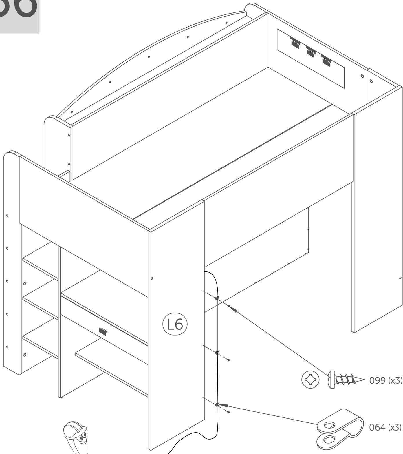
Attach the wire to the part L6 using the supports 064
