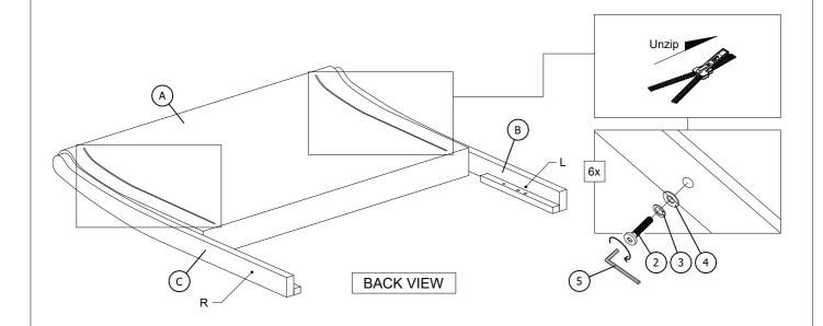
STEP 2: Assemble the Headboard Stretcher (J) with the Headboard Legs (B & C) by using Allen Key (5) with hardware (2), (3) and (4).
