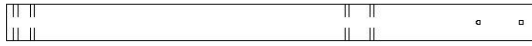
SP01 | SOPORTE DE LA VIGA DEL COLUMPIO - W4L16462 (x1) | 3 3/8"x3 3/8"x50" (86x86x1269)
