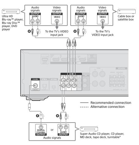
Stereo audio cable (not supplied)Coaxial digital audio cable (not supplied)
