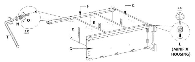
Insert the other Side Panel (Right) (D) to Bottom Panel (G). Secure the Bottom Panel (G) to Side Panel (Right) (D) with Flat Washer (O), Spring Washer (P) and JCBC Bolt (N) and tighten it with Allen Key (T). Insert Minifix Housing (L) to Side Panel (Right) (D) and follow the arrow to lock it.
