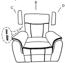
STEP 2:Install the backrest (B) by align and insert the metal bracket on the backrest (B) to the metal bracket of the seat (A).Please make sure the brackets are inserted all the way and secured into position.
