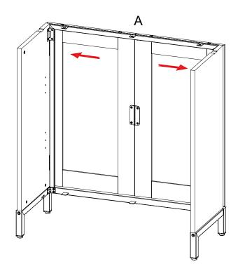
Attach Back Frame (B) to the Front Frame (A) by using Bolt (F).
